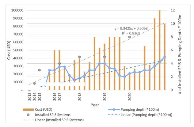
Figure 8: Installed SPIS, Related Costs & Pumping Depth (2014-2020)
